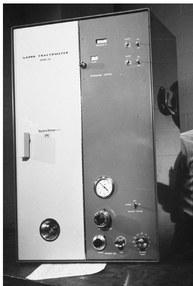
Figure 1. The Model 154 Vapor Fractometer from Perkin-Elmer introduced in May 1955. Behind the door on the left was the U-shaped column mounted on the thermal-conductivity detector block; both were in a constant temperature air thermostat. A potentiometric recorder was housed in a similar cabinet (not shown here).
