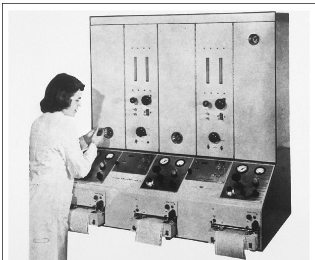
Figure 7. The Model 188 triple-stage GC from Perkin-Elmer introduced in the middle of 1957. The three units were connected in series but could also be used independently. Each unit had its own potentiometric recorder.
