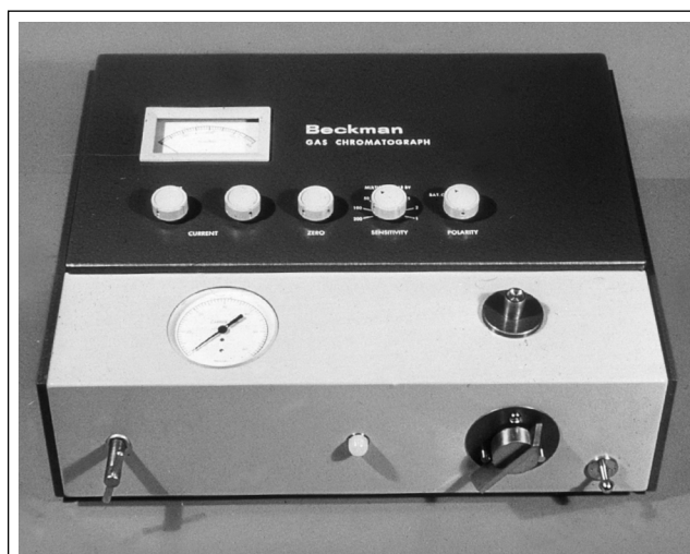
Figure 11. The Model GC-1 GC from Beckman Instruments introduced in March 1956. This instrument had a single fixed temperature control at 40^\circ\text{C} ; the Model GC-2 introduced within a year had variable temperature control possibility up to 200^\circ\text{C} .
