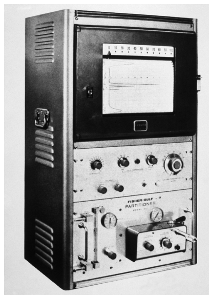
Figure 9. The Fisher Gulf Model 300 Partitioner, a slightly modified version of the original model introduced in March 1956. The box on the lower right side of the front is the micro-dipper.
