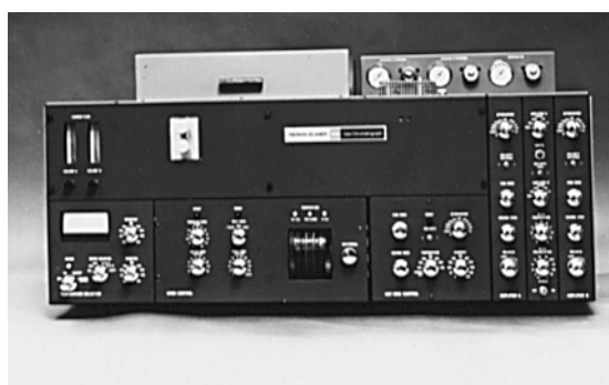
Figure 2. The Model 900 GC from Perkin-Elmer introduced in March 1967. The column oven opened on the top left; it permitted the installation of two columns (packed or capillary). Two FIDs were in the wire cage to its right; other detectors could also be installed at this place. Behind the detectors were the controls for three gases: the carrier gas, air, and hydrogen for the FIDs. The dual injection port was left of the name plate. The various knobs and dials represent temperature controls and controls for the detectors' electronics.
