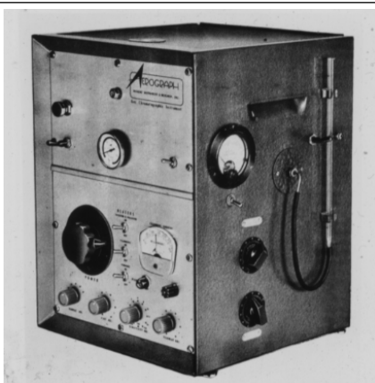
Figure 13. The Aerograph Model A-90 GC from Wilkins Instrument & Research Inc. introduced in early 1957. A bubble flow meter was attached on the side for the measurement of the carrier gas flow rate. The injection port was located just left of the name plate.
