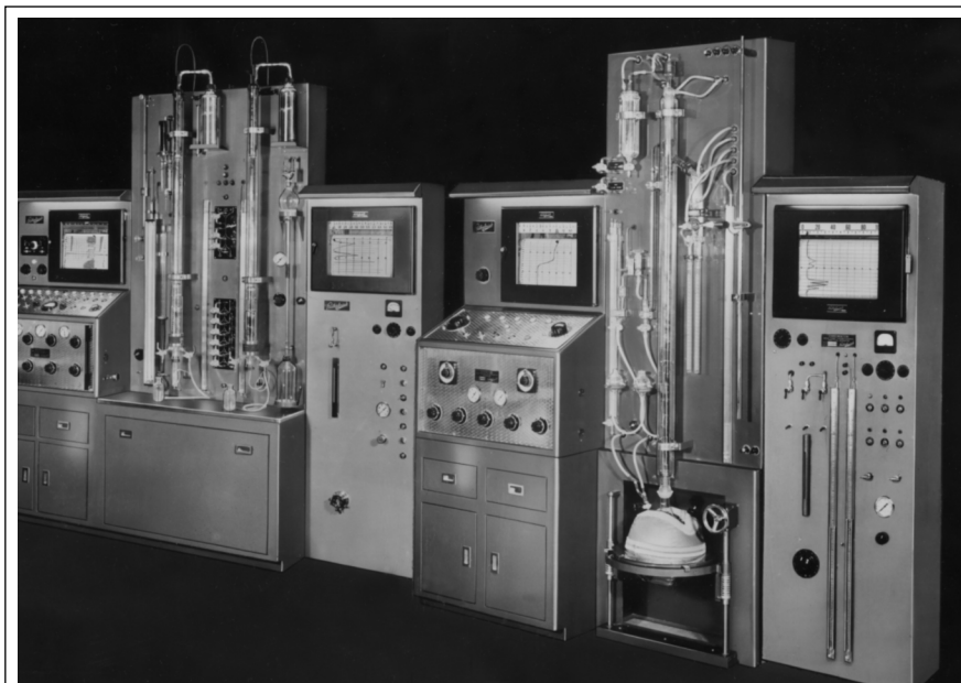
Figure 8. A publicity photo showing four instruments from Podbielniak Co.: two fractional distillation units and two Chromacon 9400 series GCs (second and fourth unit). The original Chromacon Model 9400 was introduced in December 1955.
